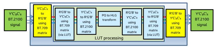
Figure 7 - Example of colour-matrix compensation within a LUT.
